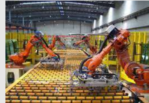
FA – Pick-and-Place by robotic arm
